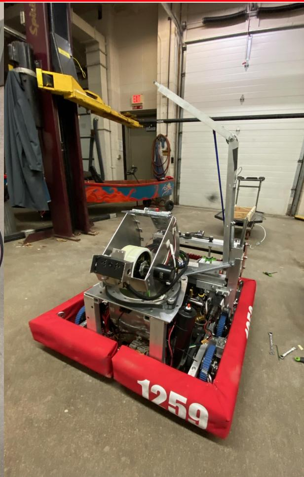
We are very proud to reveal our FRC 2020 Infinite Recharge robot, "Scorpio". Our students have worked very hard the past 8 weeks to construct this machine. Scorpio picks up Power Cells off the ground, sorts and stores 5, and can accurately shoot them from up to 25 feet away! We are on our way to Duluth, Minnesota to compete with teams from across the country.
